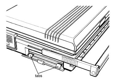
4. Lift the cover up into place and slide the release tab up to secure the cover.
